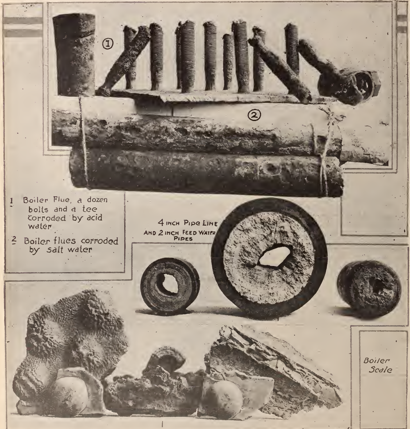
The damage done by bad water, often in an incredibly short time, can be seen by the size of the scales and the depth of the corrossions shown here
