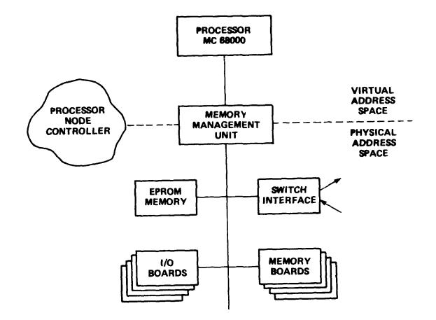
Block Diagram of Butterfly Processor Node Figure 2
