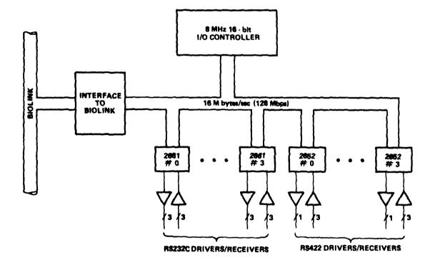
Block Diagram of Butterfly I/O Board Figure 6
