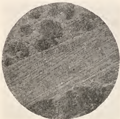
Fig. 2. Photomicrograph of longitudinal section of copper wire.
