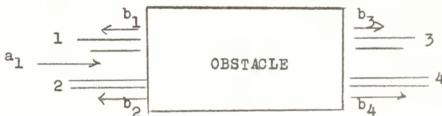
If voltage wave  $a_1$  is sent into terminal 1, then amplitude  $b_1$  will be reflected and  $b_2$ ,  $b_3$ ,  $b_4$ , will emerge from terminals 2, 3, and 4, respectively. There will be no secondary reflections into terminals 2, 3, and 4, from their respective transmission lines, provided they are properly terminated and do not couple to one another.
