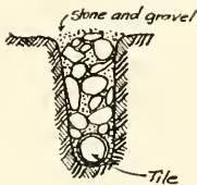
FIG. 88.—Cross-section of fill over intercepting tile drain.
