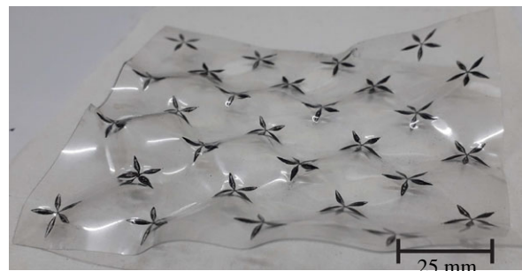
Figure 12. Patterned surface. The picture shows a textured plane, obtained by heating a flat piece of plastic which has a black and white pattern (can be doubly periodic as in this example). We can ensure that there is no large-scale bending by loosely sandwiching between two flat panes of glass while being exposed to radiation.
