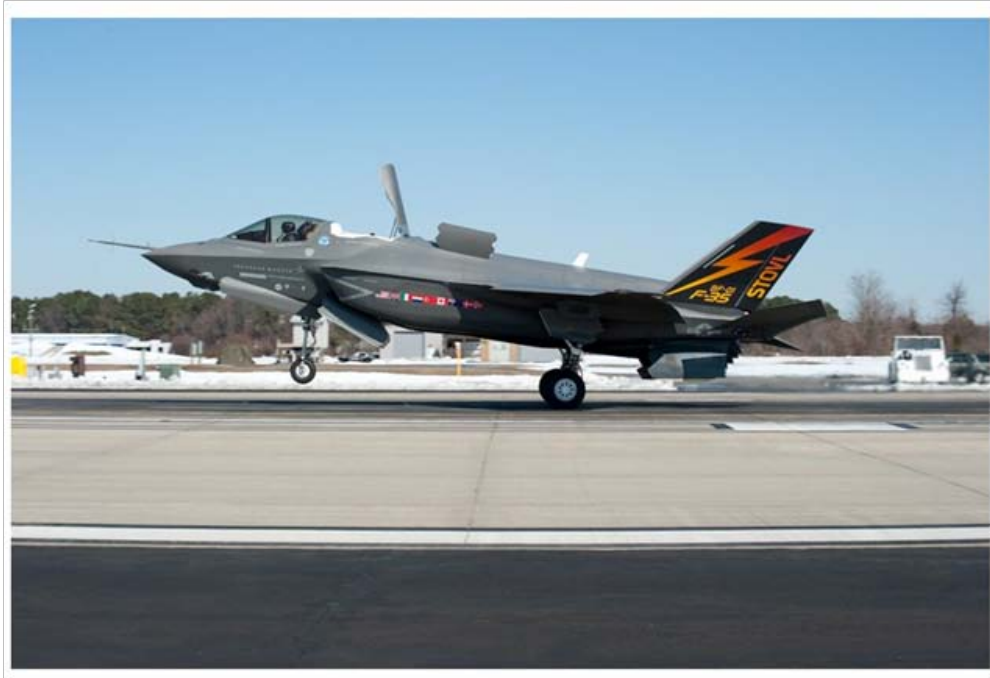
Figure 6. F-35B STOVL in test phase (From F-35 Program Office, 2010)
