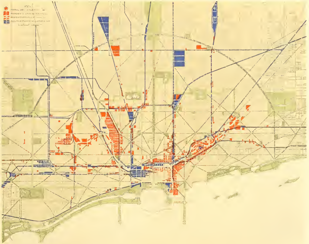
LXXXII. CHICAGO. DIAGRAM OF GENERAL SCHEME OF STREET CIRCULATION AND PARKS IN RELATION TO THE AREAS COVERED BY INDUSTRIES AND MANUFACTURES (RED). THE CENTER OF INDUSTRIES IS INDICATED BY A STAR. RAILROAD PROPERTIES AND LINES IN BLUE.
