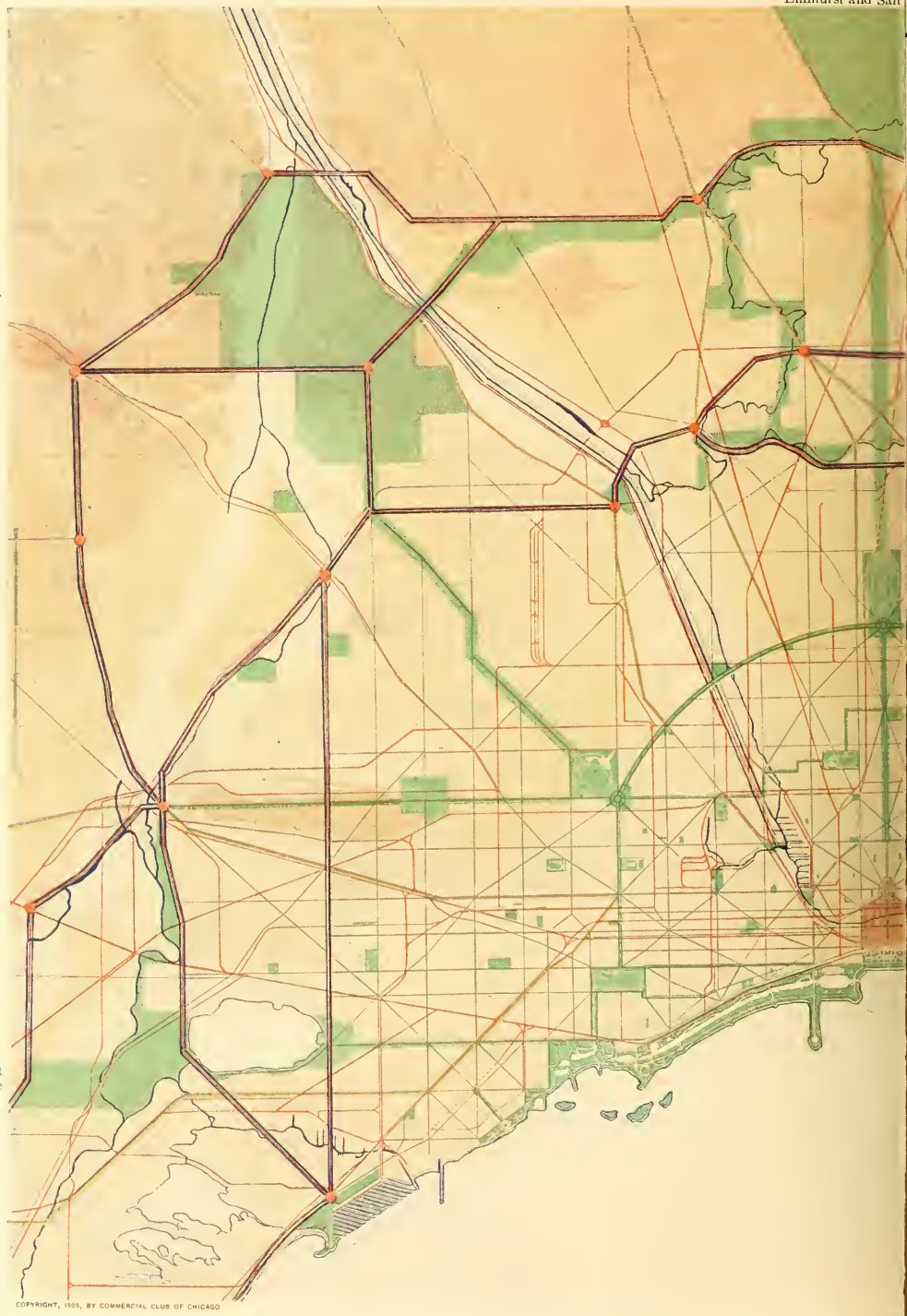
XLIV. CHICAGO. GENERAL MAP SHOWING TOPOGRAPHY, WATERWAYS, AND PARKS AND PARKWAYS ENCIRCLING THE CITY; THEY ARE PLACED IN RELATION TO THE RADIATING ARTERIES, AND INCREASE IN AREA IN PROPORTION TO THE DISTANCE FROM THE CITY. THE MAP ALSO SHOWS THE COURSE OF THE CALUMET RIVERS, AND THE LOCATION OF OUTLYING TOWNSHIPS. THE ELEVATION OF THE CITY IS SHOWN BY SHADING.
