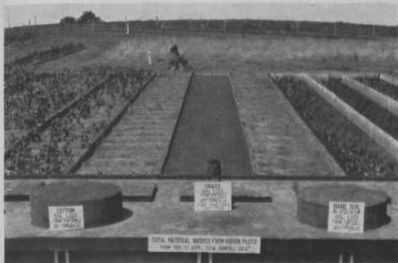
FIGURE 3.—Tests of rates of erosion under various kinds of cover and conditions are made in plots surrounded by steel guards to prevent intake of water except from overhead. The volume of the silt and run-off caught in the concrete tanks is measured.
