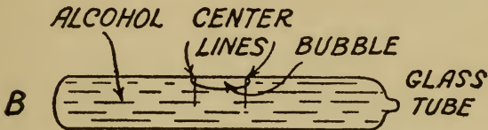
PLUMB GLASS MARKED AT ITS CENTER OR CROWNING POINT BY TWO LINES
