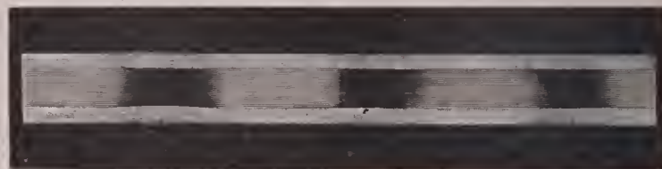
FIG. 2.—The alternate current arc, photographed on a moving plate (showing the periodic extinction of the arc).
