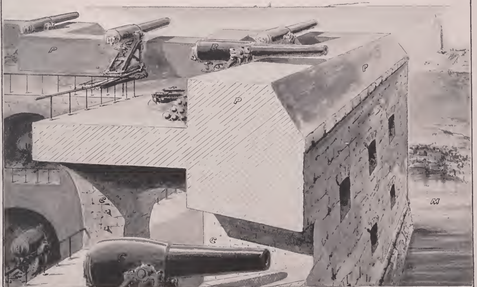
FORT. M. MOAT. P 1 PARAPET. B 1 BARBETTE GUNS. C 1 CASEMATE GUN © PORTS.
