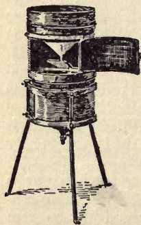
FIG. 8.—Self-recording, tipping bucket rain-gage.
