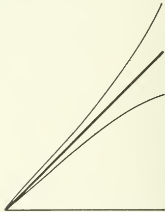
FIGURE 5.— Diagram of the effect of the injection pressure on the vein flow. The straight line represents the increasing injection pressure; the upper curve, the vein flow in the kidney; the lower curve, the vein flow in the models.
