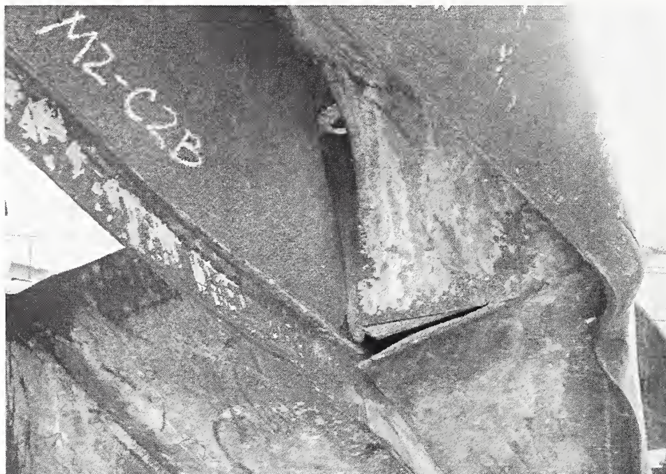
Figure 5–3. Observed impact damage in the recovered WTC exterior columns.
