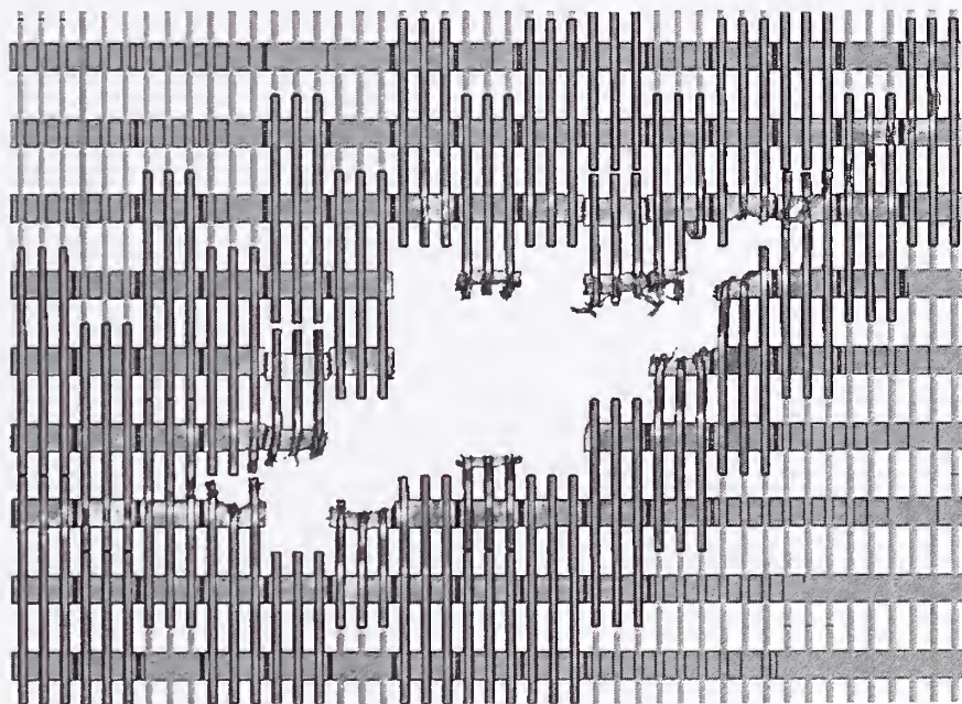
(b) Calculated damage (t=0.715 s)
