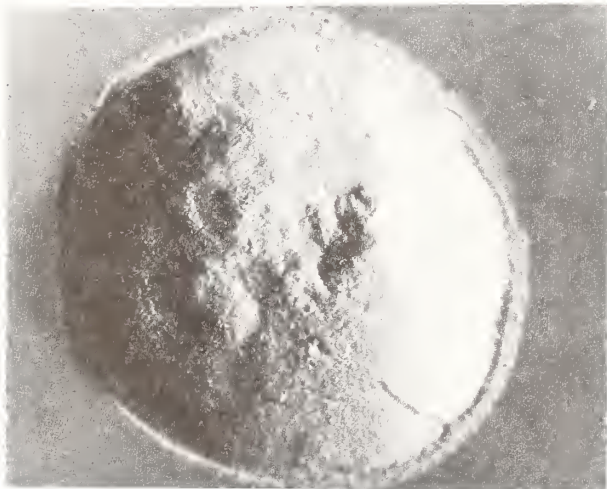
Fig. 4. Optical photograph of a 12.7-mm-diameter freeze-dried \text{U-NO}_3 sample.
