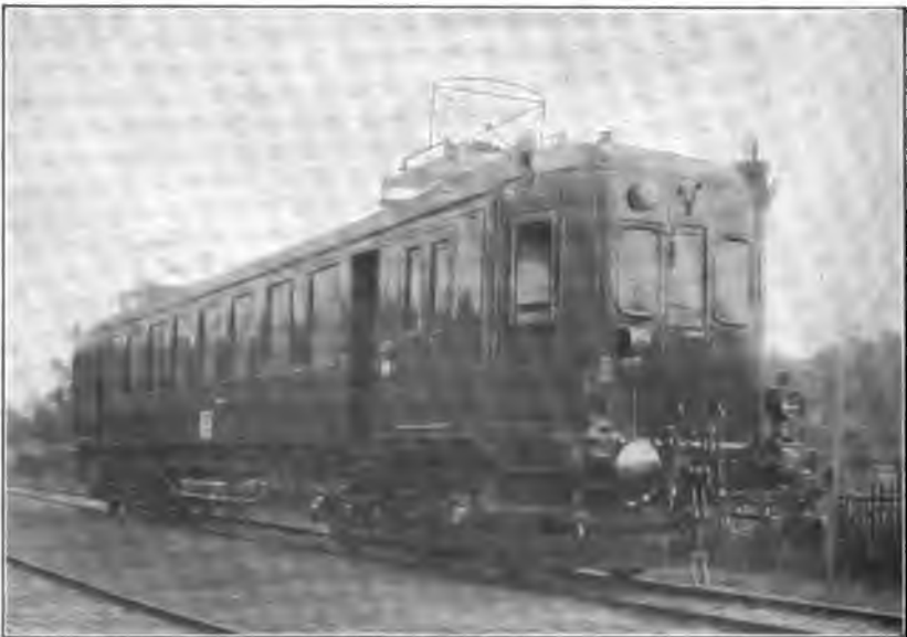
FIG. 2.—NORMAL RAILWAY CARRIAGE USED IN TRACTION EXPERIMENTS, NOW BEING MADE BY THE UNION ELEKTRIZITÄTS GESELLSCHAFT.
