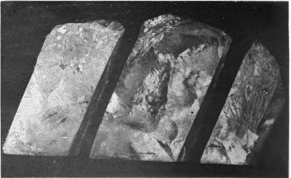
THREE PORTIONS OF THE CULLINAN DIAMOND MADE BY THE FIRST TWO CLEAVAGES, ACTUAL SIZE IN THE ROUGH
