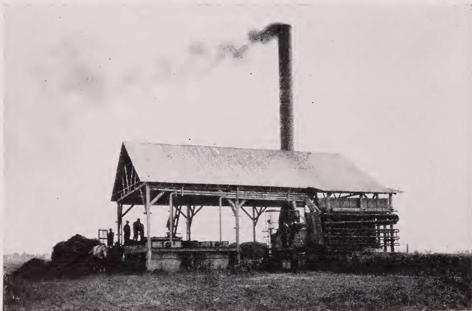
FIGURE 3.—A volatile-oil distilling unit used in the production of peppermint oil.
