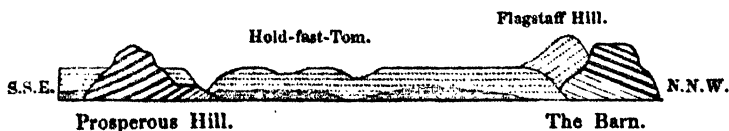
The double lines represent the basaltic strata; the single, the basal submarine strata; the dotted, the upper feldspathic strata.
