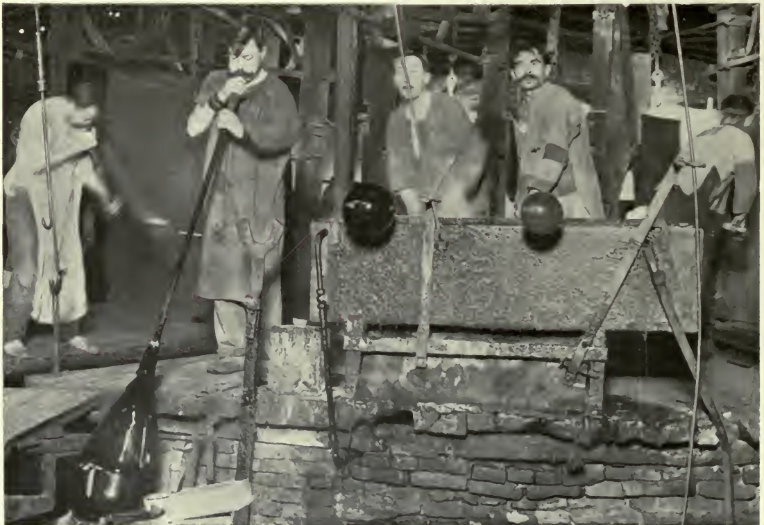
The first operation in making window panes is the blowing of glass cylinders.
