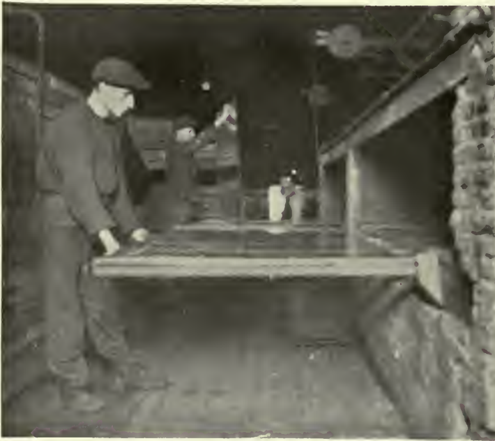
The flattened out glass as it emerges from the furnace.
