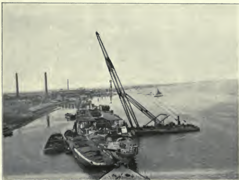
View of one of the shipbreaking yards showing the 200 tons floating-crane alongside an obsolete battleship.
