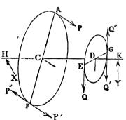
balance the forces P, Q. Then X and Y are the s if the forces P and Q, continuing parallel to themselves, were transferred to C and D.
