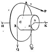
P:W::DE:CA, and therefore P:Q::CB:CA, Q being equal to W, and CB to DE: therefore W will balance P, and there will be an equilibrium. Q.E.D.
