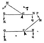
But since forces R and Q balance on the straight lever OCN, by Prop. II. R:Q::CN:CO; and since P is equal to R, and CO to CM, P:Q::CN:CM; or the forces P, Q are inversely as their arms. Q.E.D.
