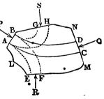
fluid, ACL, BDN become rigid; then, by Axiom 3, the forces P, Q still balance each other; but by Cor. to Ax. 2, in this case the forces P, Q are equal. And in like manner it may be shewn that the forces P, R are equal, as also the forces P, R. And R, R, R, the forces which act on the boundary of the fluid and balance each other, are the pressures on similar and equal portions of the containing vessel. Therefore the pressures exerted on all such portions are equal.
