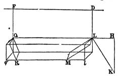
the opposite surface of the body, and cutting off the particle QR. Draw LD, QF, vertical lines, to the upper surface of the fluid. Take KL to represent the pressure on LM, and draw KH perpendicular on QL produced. And let Ll, Qq be the sections of the horizontal column by vertical planes.
