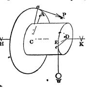
power acted, moves out of the position De into the position DE. Then the string by which the power P acts will be unwrapt from the portion aA of the circumference of the wheel, and therefore P will move through a space equal to aA. Also in the same time the string at which W acts will be wrapt upon the axle by a space equal to eE, and therefore W will move through a space equal to eE. Therefore by the definition of velocity, aA, eE are as the velocities of P and W.
