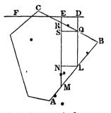
manner it may be proved that the vertical pressure downwards on the particle QR is equal to the weight of the column of fluid QDER. fore the excess of the pressures upwards above the pressures downwards on this vertical column is the
