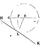
of which the center of motion is F, they will balance; being supported, as it were, by the fulcrum LF. And the sphere, which is equal to the weight A, may
