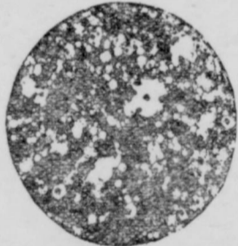
Ordinary tire rubber The white areas are "lumps" of unevenly mixed substances. Every "lump" is a weak spot that reduces mileage.
