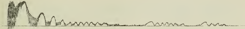
FIGURE 4. — (Eight-thirteenths the original size.) Subject, T. A. S. May 10, 1902. The exciting currents were drawn from a magneto-machine, and the contractions were recorded by means of an ergograph for the index finger. Two groups of excitations were sent in to the left abductor indicis muscle each second. Each group was formed of 17 alternating currents. A spiral spring gave a resistance of 8 ounces at the abscissa and 22 ounces at the summit of the highest contraction record.
