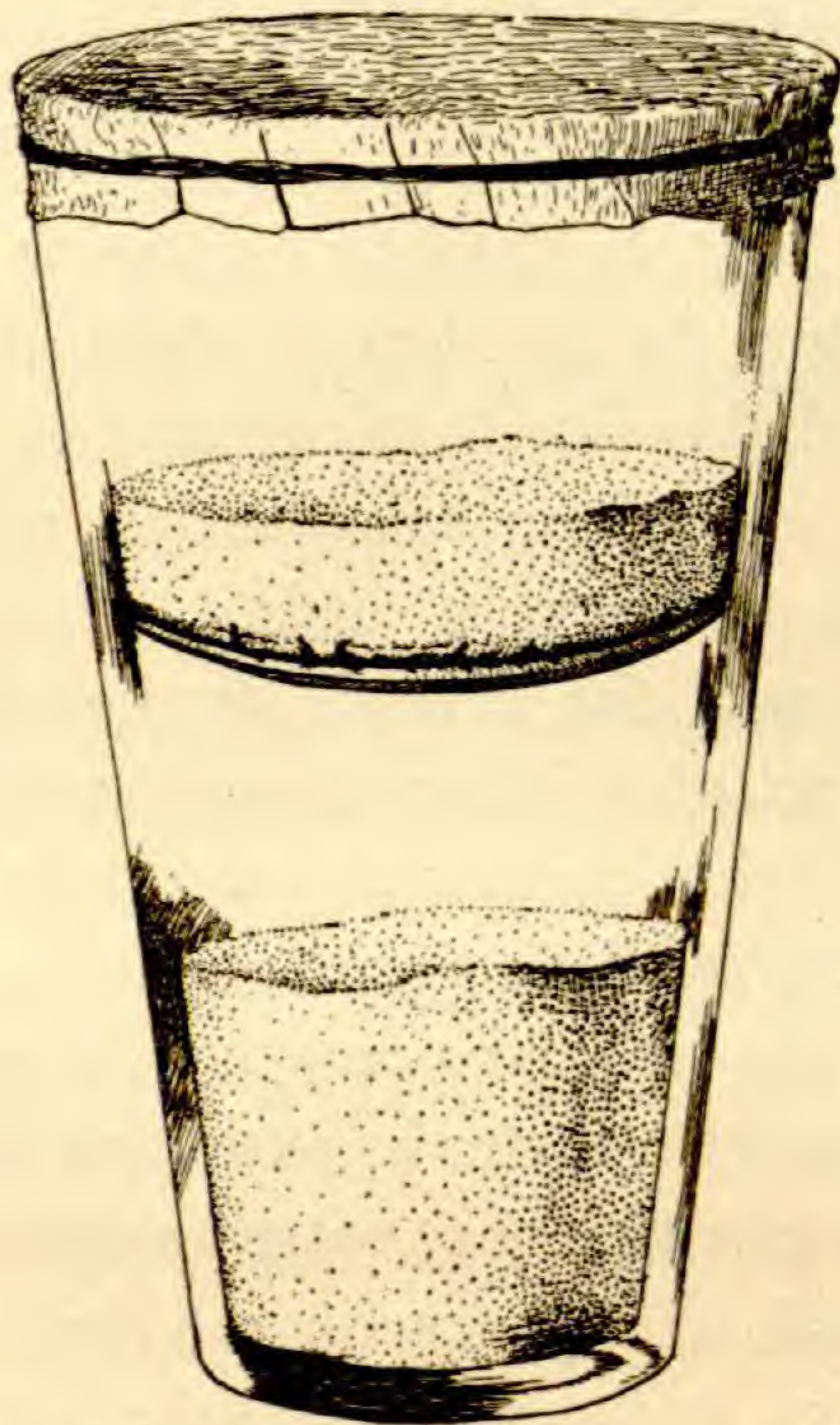
FIGURE 1. Apparatus for showing the influence of salt on vapor transfer in soils. Description in text.
