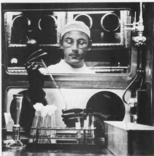
GERMS STAY PUT —laboratory researchers can work with germs without fear of infection inside this leak-proof safety cabinet developed at Fort Detrick, Md., by Army's Chemical Corps scientist-engineers. (U.S. Army Photo)
