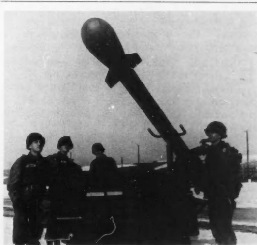
ARMY'S "DAVY CROCKETT" shown attached to a jeep. A-warhead is about size of large wastebasket and can be lifted by one man. Capable of firing atomic or conventional warheads, this weapon is culmination of imaginative efforts of the three Army engineers who will receive $25,000 award. (U.S. Army Photo)
