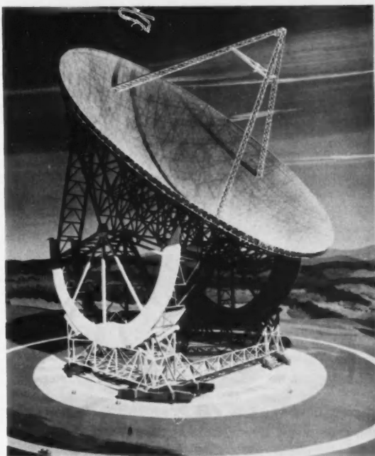
LISTEN BIG—this is an artist's conception of the 600-foot radio telescope now being erected for the Navy at Sugar Grove, W. Va. Conceived by and to be instrumented by Naval Research Laboratory scientists, the 30,000-ton structure, over 7 acres in area, will provide the U.S. with one of the world's foremost tools with which to study outer space, enabling scientists to listen in on space sounds at the "edge of the universe"—38 billion light years away. (Official U.S. Navy Photo)
