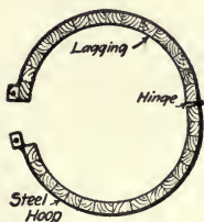
Fig. 189.—Form for Circular Column.
