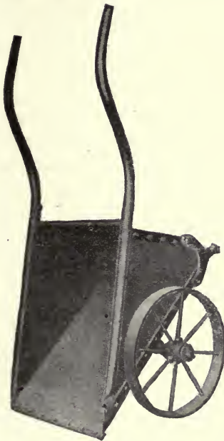
Fig. 17.—Forward Dump Charging Barrow, Ransome Concrete Machinery Co. mixer engine is an excellent arrangement. A prong riveted to the rear face of the barrow and projecting downward is "caught into" the chain, which pulls the barrow to the top, the man following to dump and return for another load.
