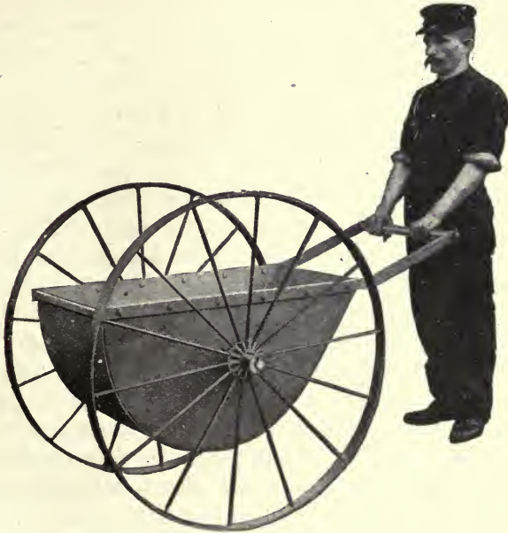
Fig. 12.—Two-Wheeled Ransome Cart for Hauling Concrete.
