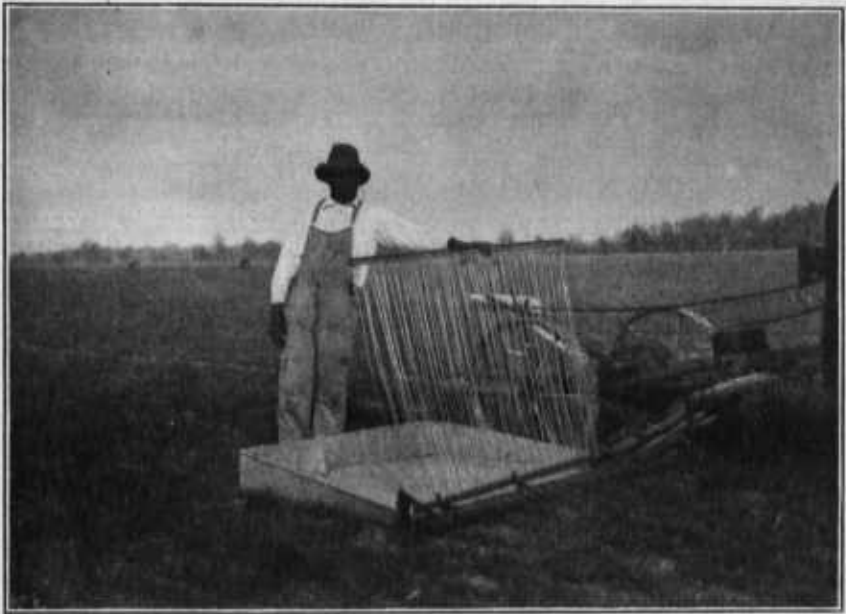
FIG. 6.—Lespedeza pan, with top raised to show wires or rods between which the seed falls into the pan when the crop is harvested.
