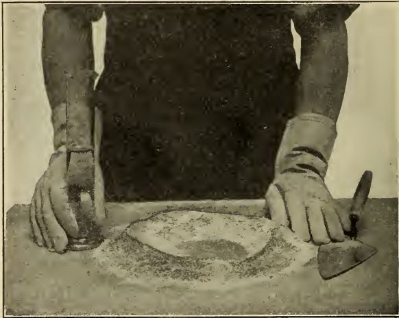
FIG. 50.—Making Briquettes—Adding the Water.
