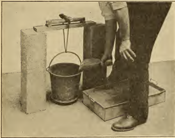
FIG. 123.—Illustrating the Method of Making Transverse Tests Without Apparatus.
