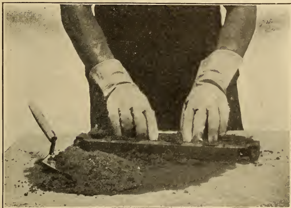
FIG. 52.—Making Briquettes—Filling the Mould.
