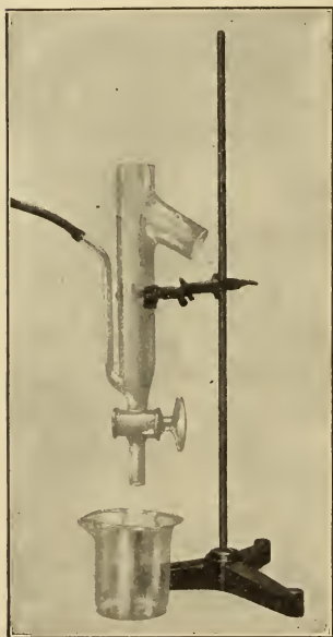
FIG. 29. — Apparatus for Determining Fineness by Washing.
