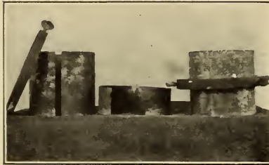
FIG. 110.—A Simple Form of Cylindrical Mould for Concrete.
