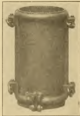
FIG. 109.—Mould for 6-in. Cylinders of Concrete.
