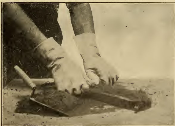
FIG. 53.—Making Briquettes—Compacting the Mortar.
