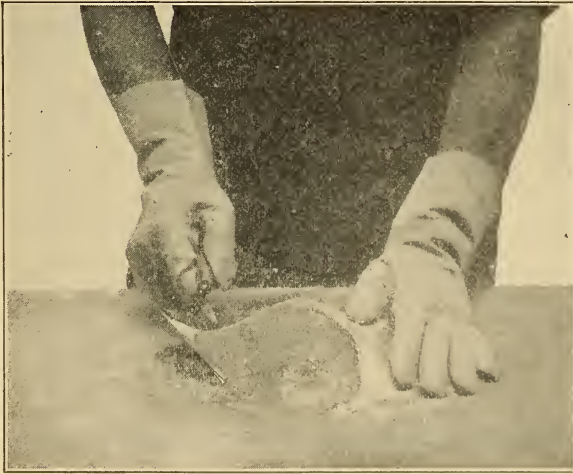
FIG. 49.—Making Briquettes—Mixing the Dry Ingredients.
