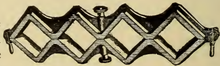
FIG. 111.—Gang Mould for 2-in. Cubes.
