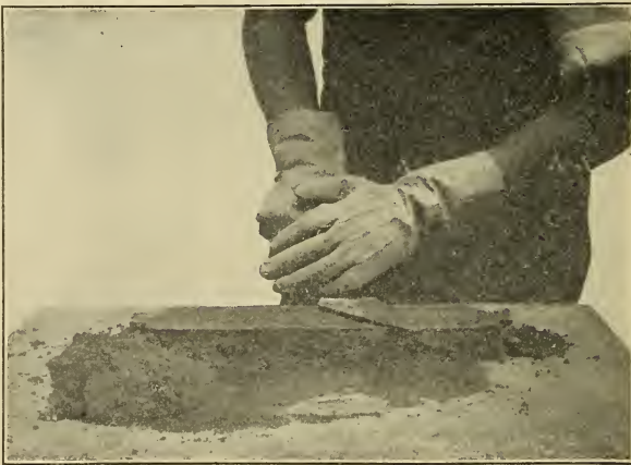
FIG. 54.—Making Briquettes—Troweling the Surface.
