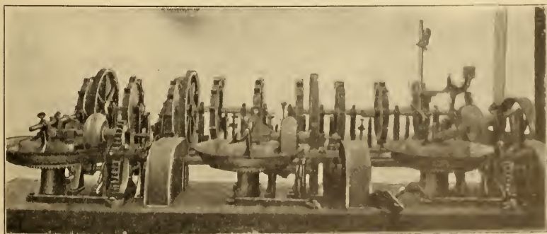
FIG. 63.—A Battery of Mechanical Briquette Formers in the Royal Testing Laboratory at Berlin, Germany.
