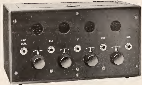
THE WINKLER DETECTOR AND 3 STAGE AMPLIFIER TYPE 4B.
