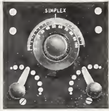
No. 47489 Simplex Vario-Coupler, Showing Front View of Panel Mounted Type
