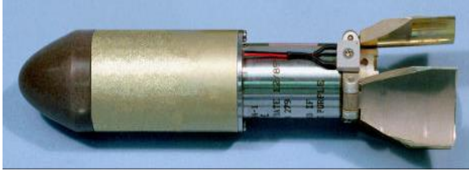
Figure 5. Prototype RT-1489/ALE GEN-X Decoy and Canister. Source: Koppenberger (2017).
