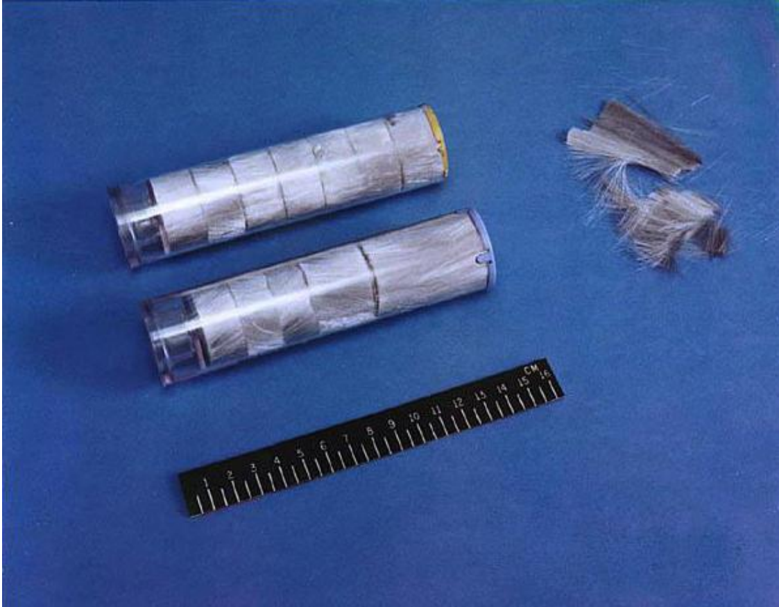
U.S. Navy RR-144A/AL training chaff is shown on top and RR-129A/AL Chaff shown on bottom. Notice the different length in the RR-129A/AL compared to the uniform lengths in the RR-144A/AL. The fibers on the right show the dipoles outside of the canister.
