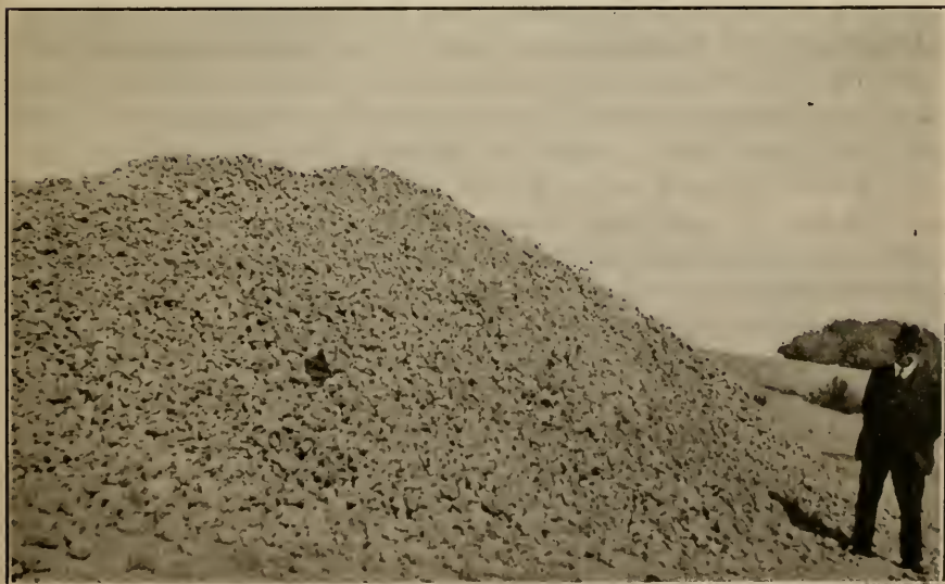
Brand & Stevens' pumice, Imperial County. Thirty-ton dump of pumice, selected for grinding, awaiting shipment. Shows average size of material obtained. Photo by Emile Huguenin.
