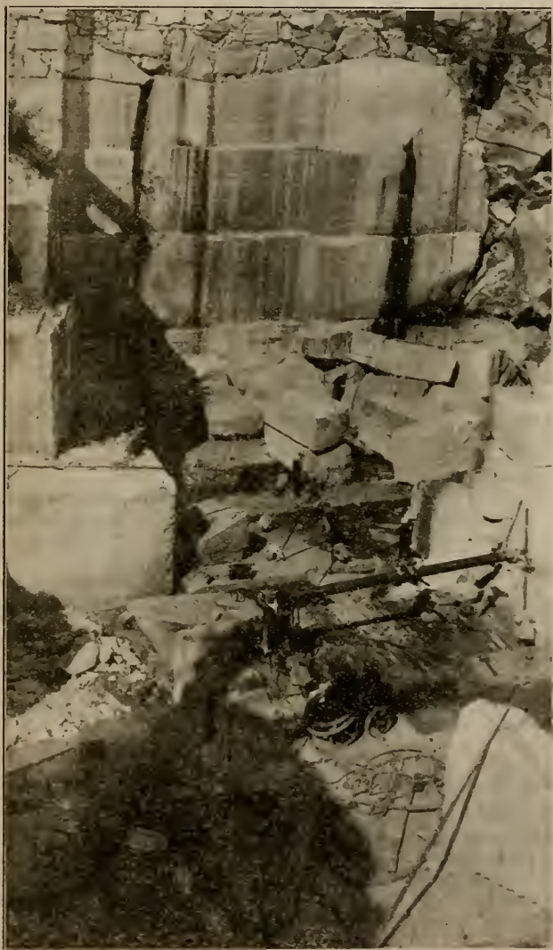
In quarry of Columbia Marble Company of Columbia, Tuolumne County, showing channeled faces. Photo by C. A. Logan.
