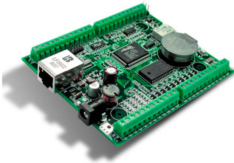
Figure 18. BL2000 Microcontroller (From [12])
