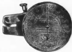
The Ashcroft Thickness Gauge
