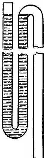
Fig. 145. S-trap, with seal 6 feet deep, which lost its seal, tested on the same apparatus.
