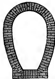
Fig. 50. Section of Egg-Shaped Sewer.
