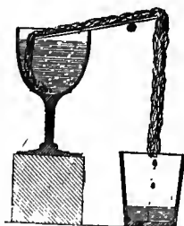
Fig. 286. Capillary Action with Horizontal Extension.
