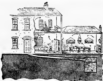
Fig. 598. Addition to a house built over an unsuspected cesspool.
