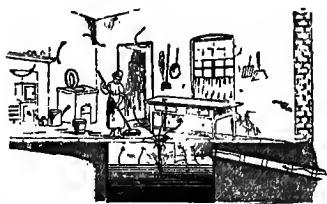
Fig. 633. Dish stone in scullery untrapped, and opening direct into a rain water tank, with overflow into drain.
