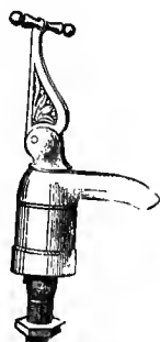
Figs. 369 and 369a. Section and Perspective View of the Writer's Slow Closing Faucet.
