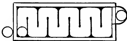
Fig. 163. S-traps placed horizontally.
