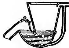
Fig. 414. Section of the English Siphon Jet Patent of 1842 of Thomas Smith.
