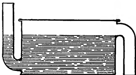
Fig. 146. Pot trap nine inches in diameter.
