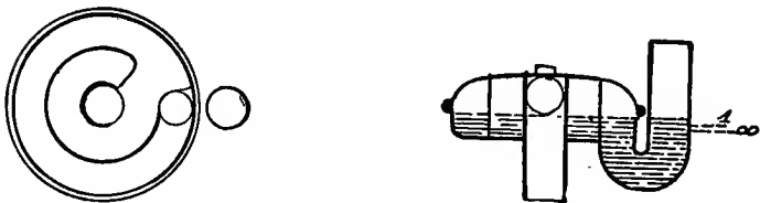
Figs. 197 and 198. Spiral Basin Trap.
