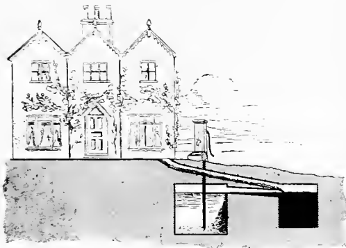
Fig. 593. New Vicarage Cesspool overflowing into a Tank.
