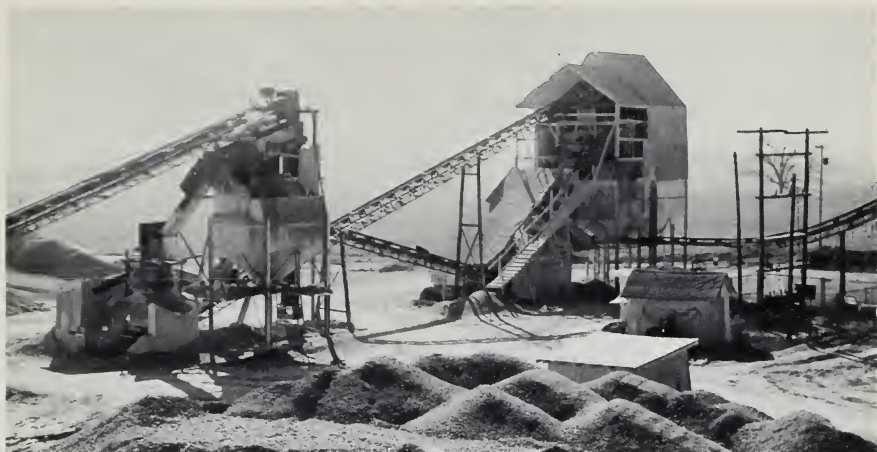
Big quarry near Corydon uses 500-horsepower connected load to power its digging and crushing work. It produces architectural and road-building stone.
