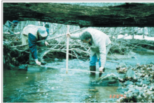
Mean annual flow can be determined by application of known regression equations to simple stream measurements.
