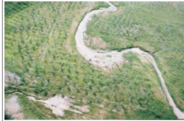
Small alluvial fan in lower left at base of small channel. Water flows by sheet flow to channel on the right. Does jurisdiction continue in absence of continuous OHWM?
