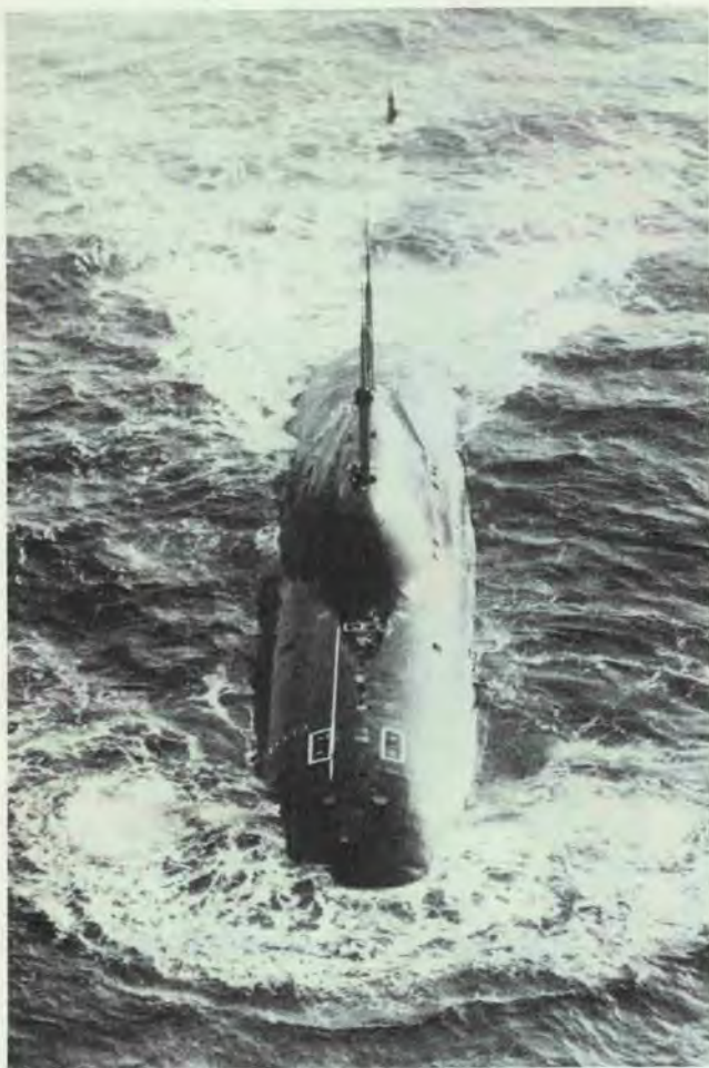
The Soviet Navy's nuclear-powered, deep-diving, titanium-hulled ALFA-Class torpedo attack submarine is the world's fastest, with submerged speeds of over 40 knots.
