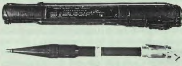
Soviet RPG-18 Antitank Rocket, a close copy of the US LAW antitank weapon.
