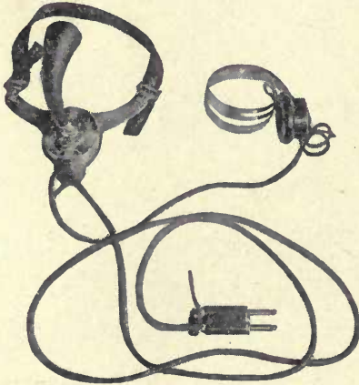
Fig. 272. Operator's Talking Set
