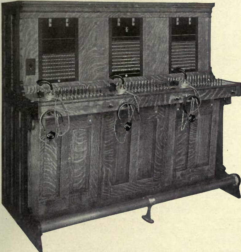
Fig. 329 Three-Position Lamp Board
