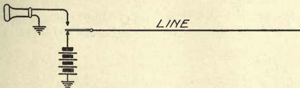
Fig. 657. Telephone Test for Capacity
