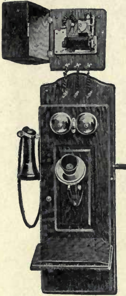
Fig. 191. K. B. Lock-Out Station
