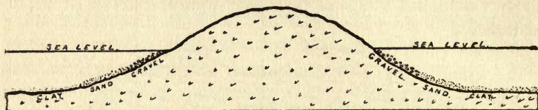
FIG. 7.—Diagram to illustrate the theoretical disposition of sediments about an island.
