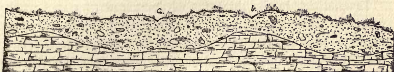
FIG. 32.—Diagrammatic section showing relation of drift to underlying rock, where the drift is thick relative to the relief of the rock. a and b represent the location of post-glacial valleys.
