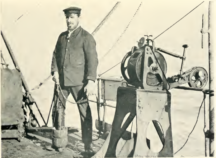
FLETCHER WITH THE DRIVER LOADED READY TO TAKE A SOUNDING
