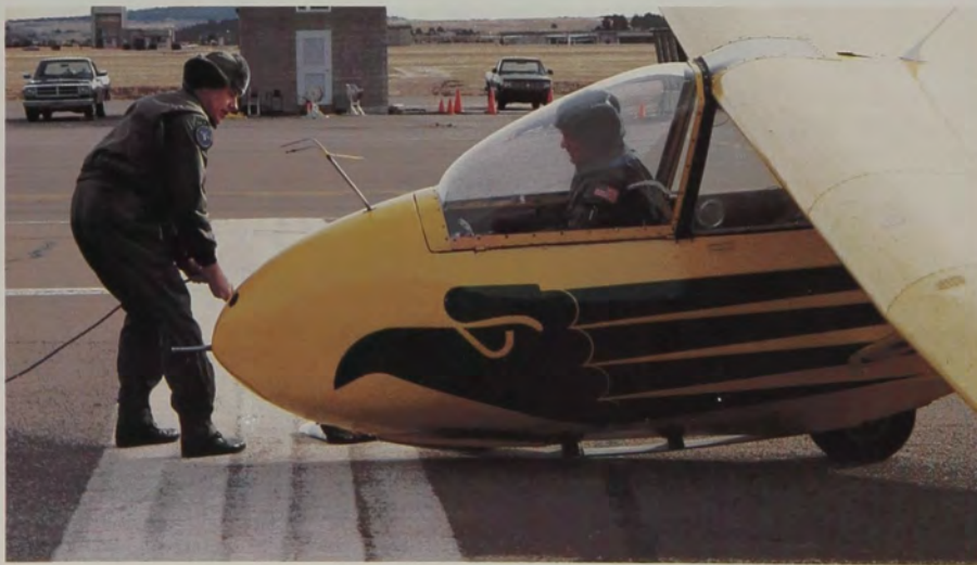
Hitching a ride. This instructor pilot better known as the I.P. checks the tow rope to make sure that it's hooked up properly. Photo by C. Grosjean.
