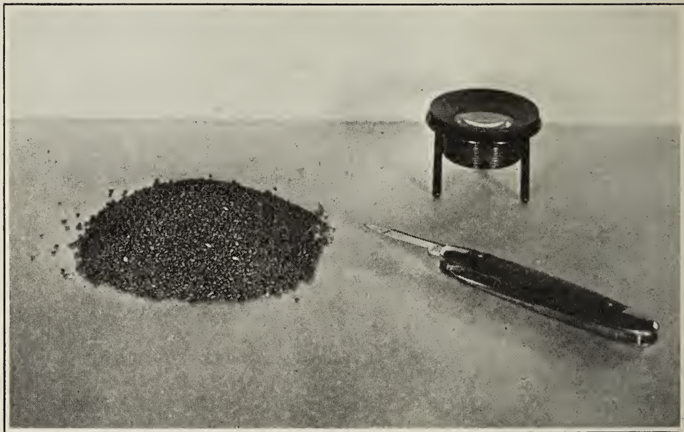
FIG. 2.—The seed to be tested as to purity is spread out on a sheet of paper. A knife and simple tripod lens are all the apparatus necessary to separate the seed into pure seed, weed seed and other crop seeds, and inert matter.
