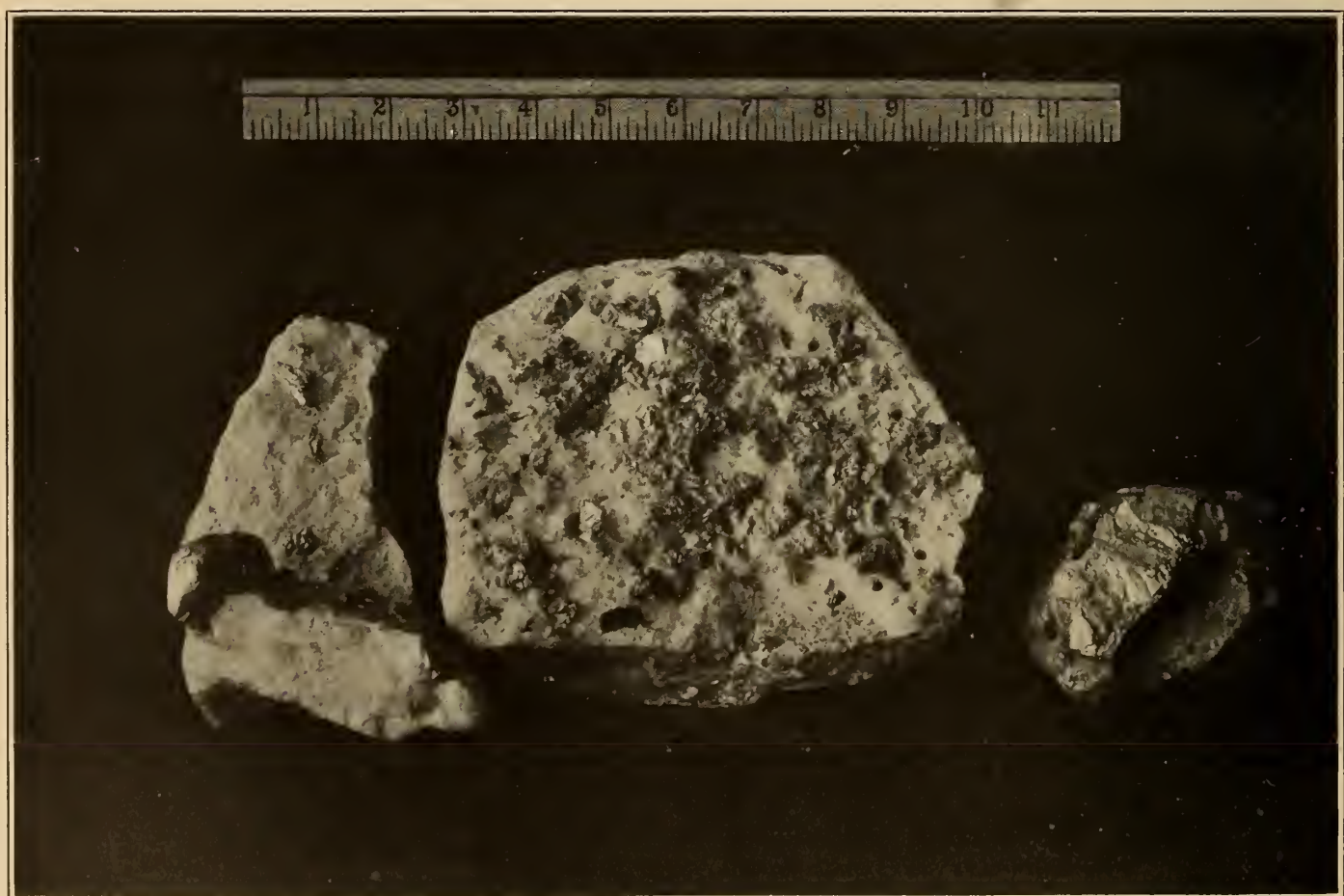
FIGURE 2.—MOLYBDENITE CRYSTALS IN QUARTZ
