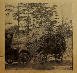
In pulling a half-ton load, the gasoline consumption of the car is increased by about one seventh
