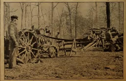
A tractor furnishes plenty of power to send a circular saw through hard knots without loss of speed
