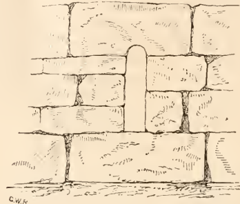
Fig. 146. Outside elevation of a slit window.
