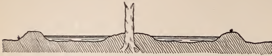
FIG. 23.—Method of grading interior of basins to prevent water coming in direct contact with trunk of trees.
