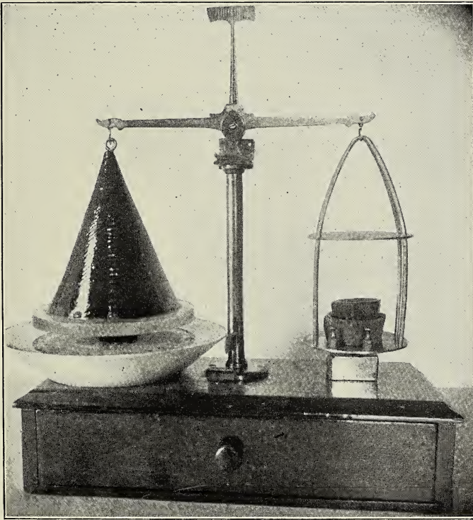
Method of cone suspension in apparatus for finding the cohesion of water.
