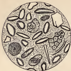
Fig. 14. — Slice of arenaceous and oolitic limestone from the Carboniferous series of Shap, Westmoreland; magnified. The section also exhibits Foraminifera and other minute fossils. (Original.)
