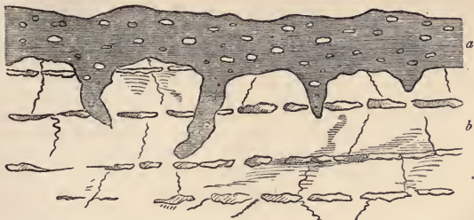
Fig. 18.—Section showing strata of Tertiary age ( a ) resting upon a worn and eroded surface of White Chalk ( b ), the stratification of which is marked by lines of flint.
