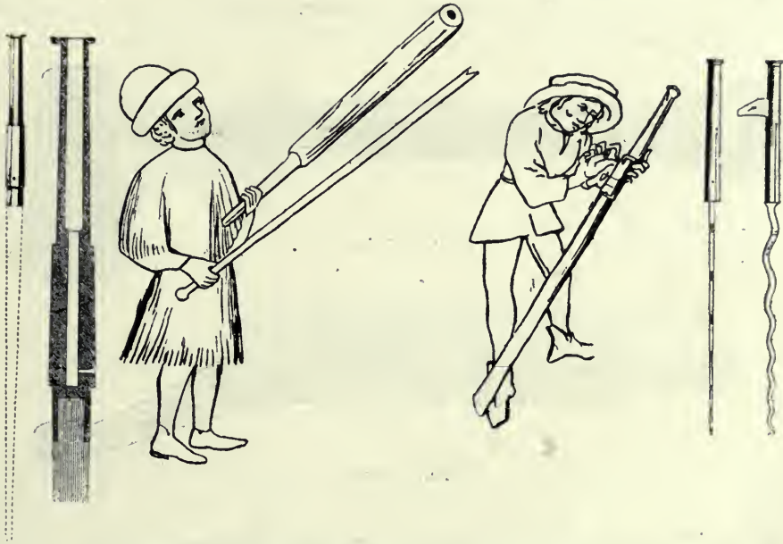
Early Hand-guns, showing Methods of handling them, as illustrated in contemporary MS. ; and a Sectional View of Gun, showing its Construction.
