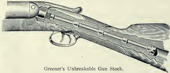
Greener's Unbreakable Gun Stock.
