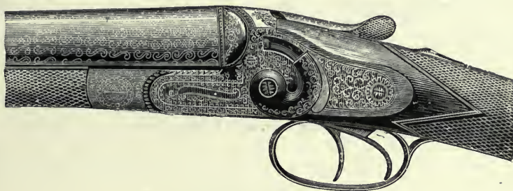
The Semi-hammerless Gun.
