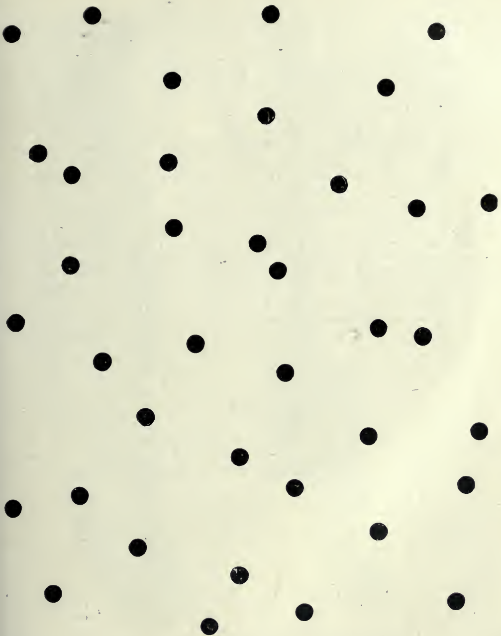
Diagram of 10-bore Full-choke, with No. 6 Shot, at 40 yards.
