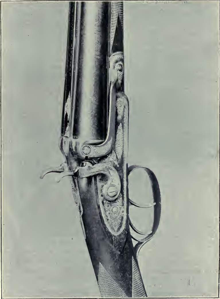
Needham's Snap-action Mechanism,
