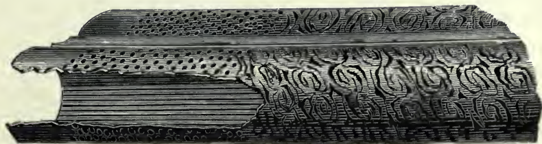
Grooved and Perforated Shot Barrel.
