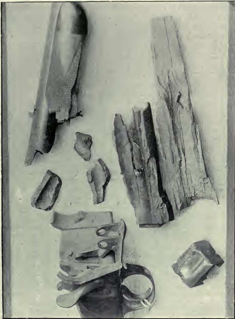
"Express" Rifle burst with Fine-grain Powder.
