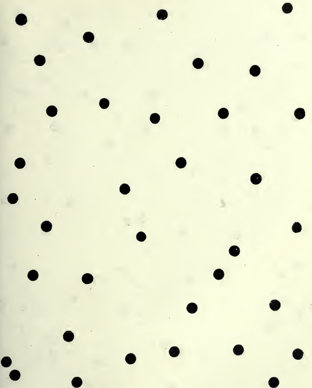
Pattern of 12-bore Choke, with 1\frac{1}{8} oz. No. 6 Shot, at 40 yards.
