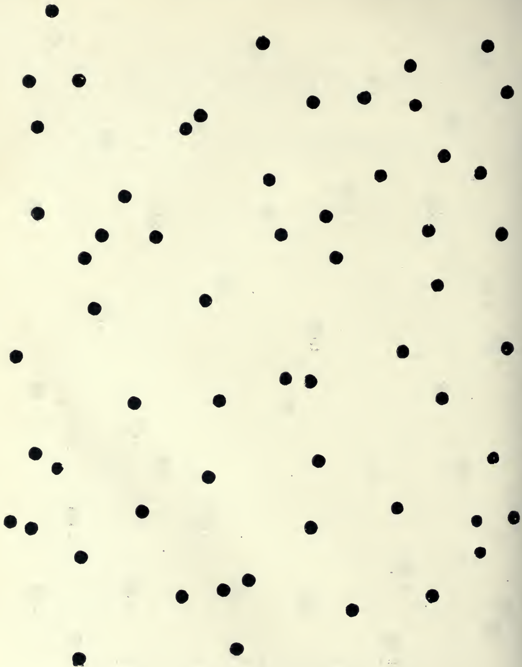
Diagram of 12-bore Full Choke, and No. 8 Shot, at 40 yards.
