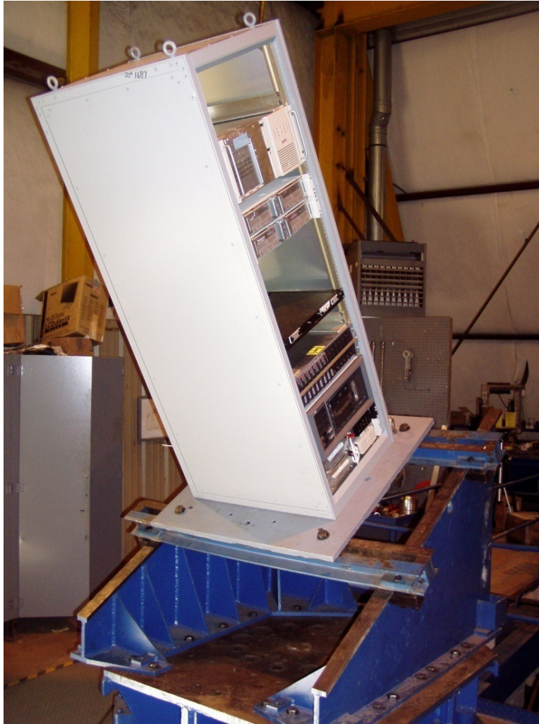
Figure 28. Medium Weight Shock Machine. Source: [104].
