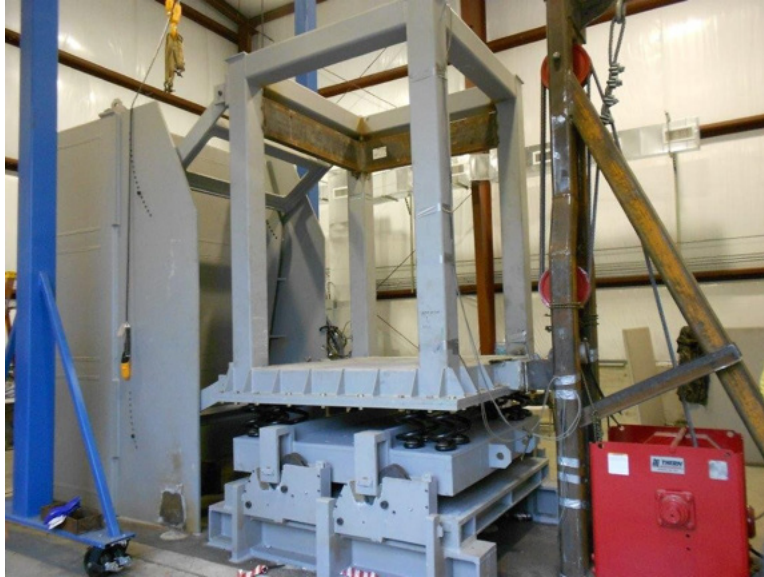
Figure 31. Deck Shock Simulator Module. Source: [107].
