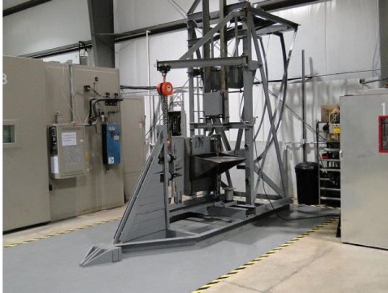
Figure 27. Light Weight Shock Machine. Source: [103].
