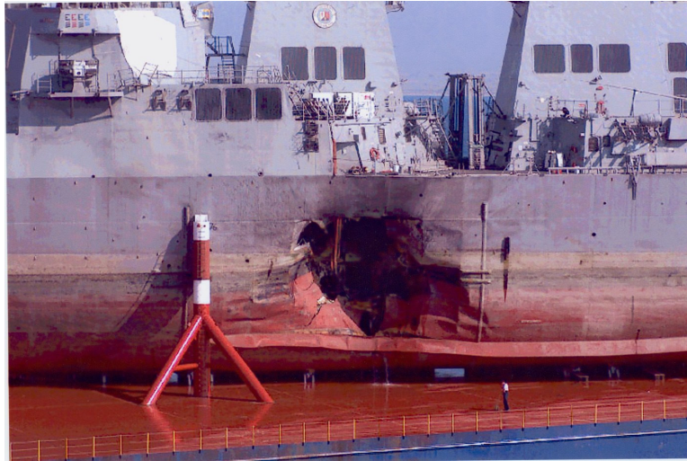
Figure 3. Holing Visible on the Port Side of USS Cole (DDG 67) During Heavy Lift. Source: [27].
