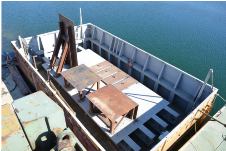
Figure 56. Floating Shock Platform with DSF Installed. Source: [130].
